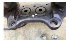
2. Temporarily put the insert in the caliper and line them up as shown. The outer alignment marks should be in a straight line with the other. The marks 90 degrees to the outter will line up to the casting edge of the Caliper.
