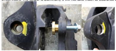
4. Align insert and use a shop press or C clamp to press each insert into caliper. A mallet will work too just be sure to not allow the insert to misalign. The inserts should be a light press fit.
