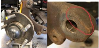
6. Install Caliper (with no rotor) to spindle to verify insert alignment. Install rotor, caliper, and pads. Tighten to factory 94-04 caliper torque specs. Customer may choose to sand or machine the outside edge of the brake pads so they do not sit proud of the rotor, however this is preference of installer and not necessary.
