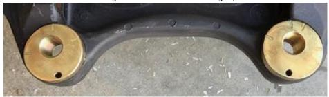
5. Install rotor shim. Depending on age and rust of spindle, the corners may need slightly cleaned up with a flap disk or wire wheel to ensure no interference to the mounting face of the caliper, check/fix all 4.
