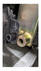
3. Bolt bracket to spindle. The lock nut should be on the ball joint side and bolt head on rotor side. Tighten to factory caliper bracket specifications.
