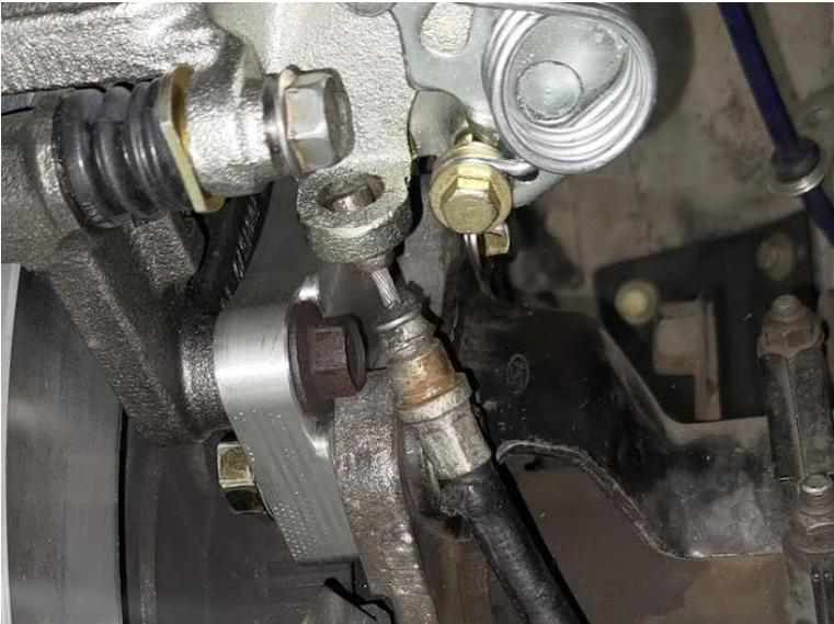
*Figure 6 - caliper bolts clearing SRA Ford Cobra bracket "ears"*
